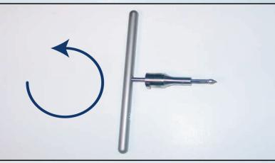
**Step 5** - After the screw has been removed, dispose of the screw and extractor tip. Extractor tips are **single use only**.
