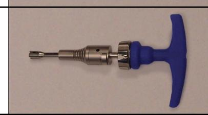
**Step 4** - Set the extractor tip over the shaft of the broken screw and TURN THE HANDLE COUNTER CLOCKWISE. The extractor tip will cut into the screw and then back the screw out of the bone.
