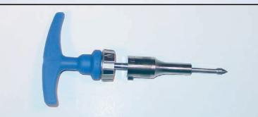
Step 4 - Set the tip of the extractor into the socket of the stripped screw and TURN THE HANDLE COUNTER CLOCKWISE. If using the ratcheting T-handle, turn the sleeve on the handle in the correct direction for counter clockwise locking of the extractor. The extractor will bite into the screw and then back the screw out of the bone or plate with continued torquing.
